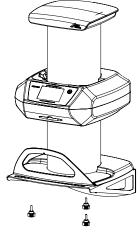
• Use the knurled screws to fix the VistaScan View securely onto the wall mounting bracket.
