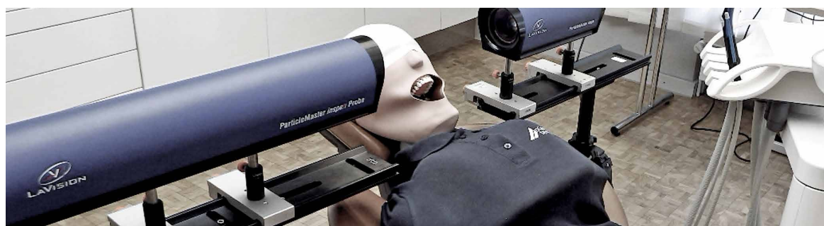
Measurement setup with unit for background lighting on the left and lens on the right, close to the head. The optical frame is located 5 cm above tooth 11.
