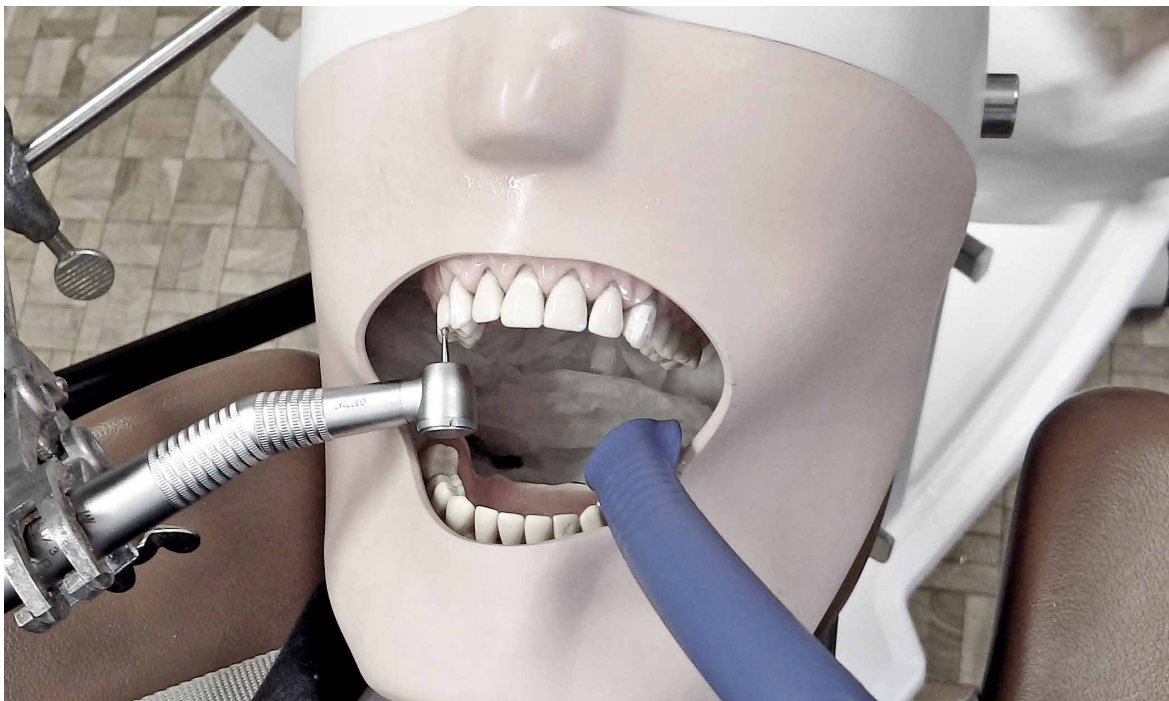
Examination setup with sub-optimal suction position using the universal cannula Protect suction cannula. The flow rate was set by means of the slide on the suction handpiece
